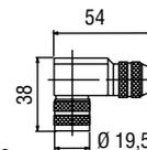
6 pin 90° female connector M16 insert adjustable in 45° positions
