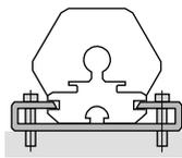
Mounting clamp with screws M5x20
